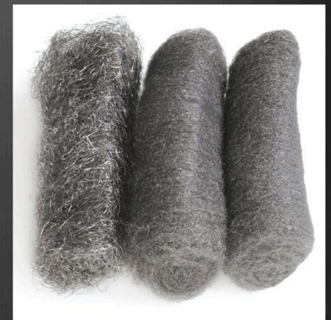
Why to use steel wool as a vibration damper viscoelastic material ✓ Damping varies with temperature > porous metallic material ✓ Tangled metal wire material - Difficult to fabricate  $\checkmark$  Metal swarf
